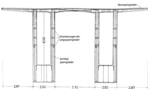
Fig. 5: cross section of Finsterwalder's longitudinal and transverse prestressing
