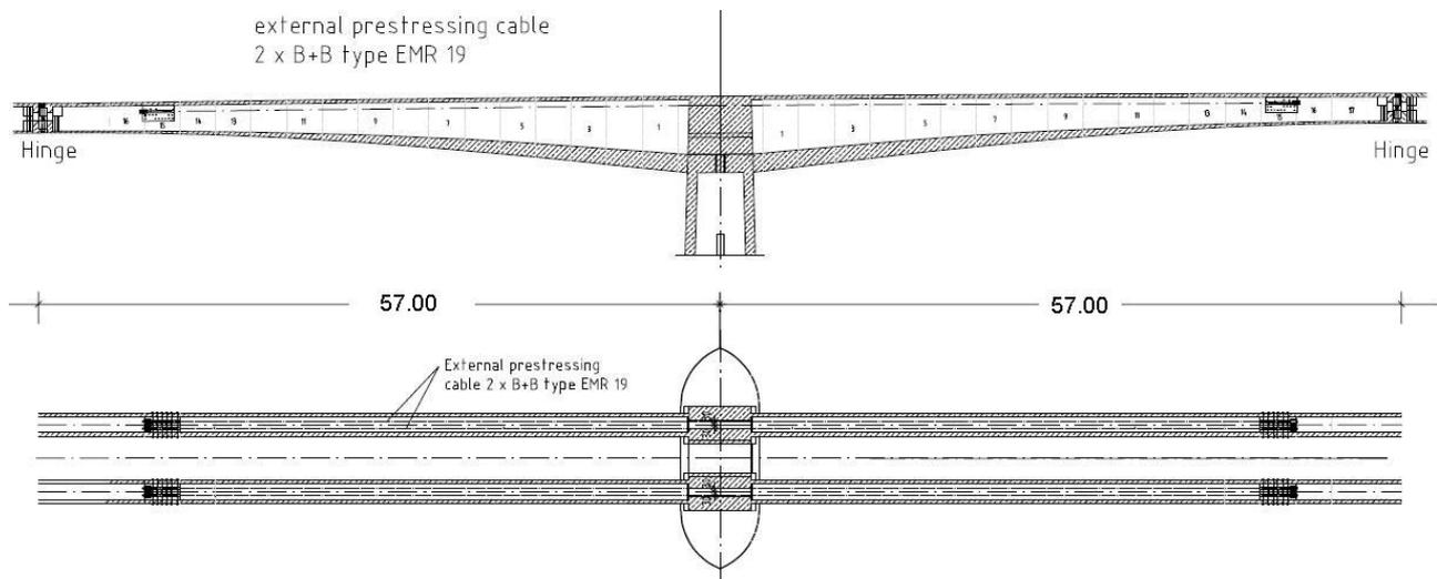
Fig. 6: Reinforcing the cantilever beams with external longitudinal tendons
