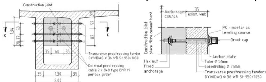
Fig. 07: Detail of the anchorage of the external additional prestressing tendons Left: Cross section of a hollow box at end of the cantilever Right: Detail of the anchorage block with transverse prestressing bar St 950/1050)
