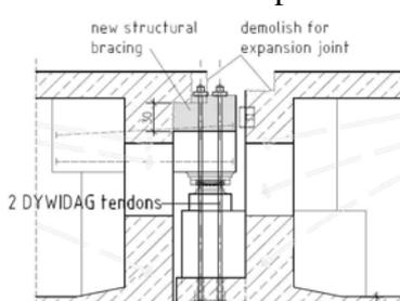
Fig. 8: Hinge in the crown with prestressing anchor and spherical bearing
