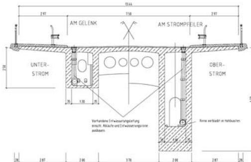
Fig. 3: Cross section of the centre bridge
